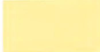
Colortherm® Yellow 10 offers increased heat stability of approximately 20 °C, relative to standard iron oxide yellow pigments, due to a post-treatment with inorganic oxides.
